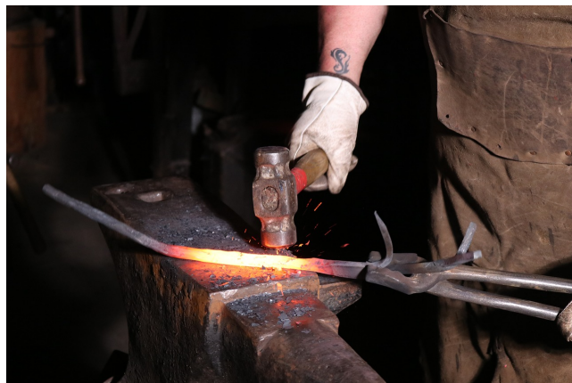
Figure 1: This metal visibly glows almost white because it is hot and k_B T \approx 2 eV. You can see that parts of it which are a bit cooler glow red, and other parts don't glow at all in the visible spectrum.
